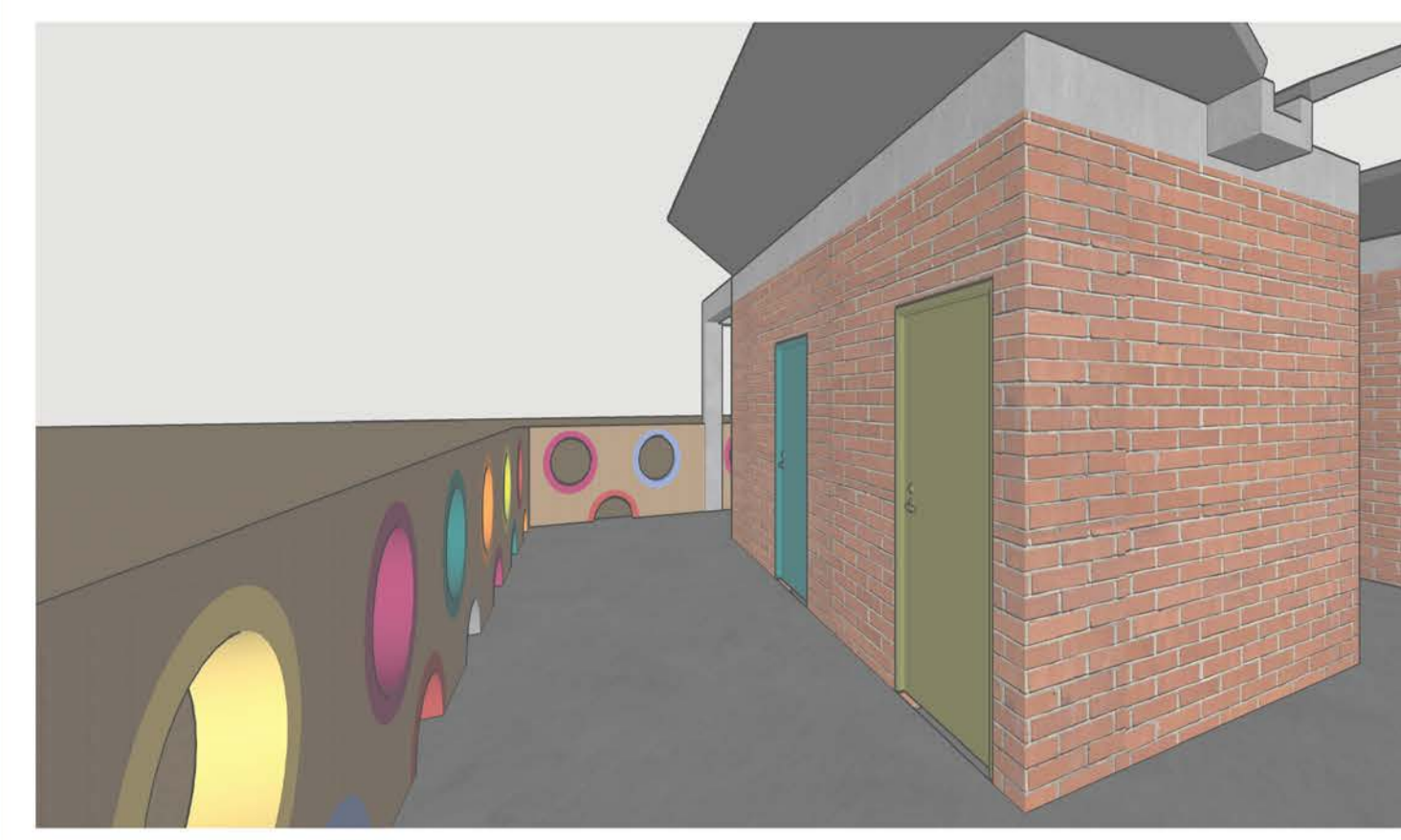
- Combined toilets for all age groups and visual connectivity for safety - Playful compound walls for visual connectivity and child development
