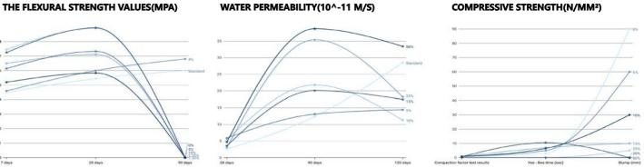
Although the compressive strength is lowered by using seashells as cement replacement, concrete made with inclusion of shell ash still have acceptable strengths for various structural. The optimum substitution level of cement with seashell ash was found to be 5-10%. Using seashell cement clearly enhances the splitting tensile and exural strengths of concrete by enhancing the bond at the cement paste interface.
